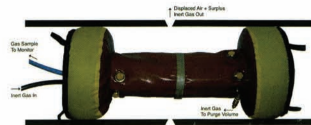
Fig 4: Cross section of inflated Quick Purge system inside pipe showing gas paths and oxygen sampling port
