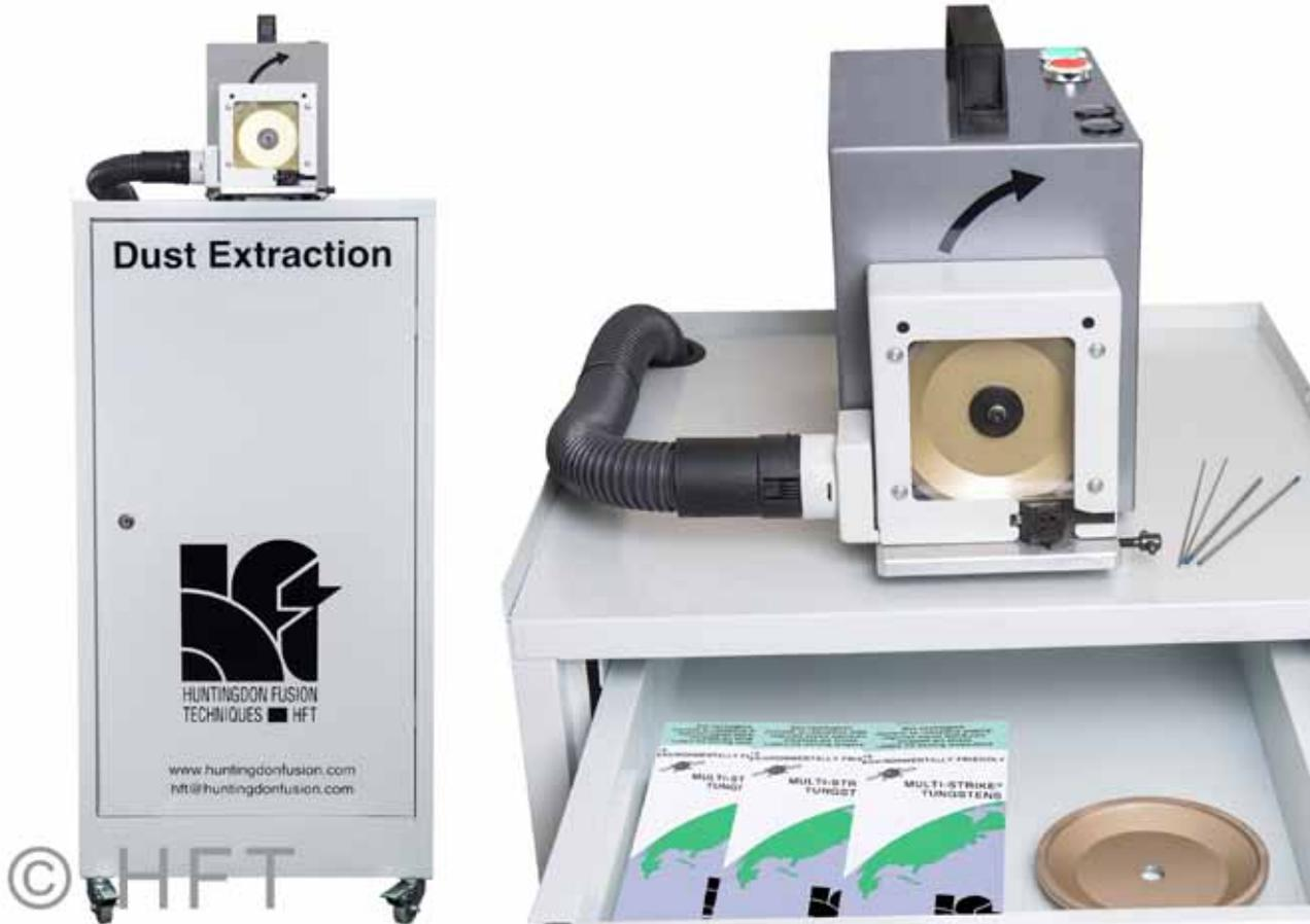
A new **Mobile operating station with dust extraction system** for the **TEG-1000 Tungsten Electrode Grinder** has now been brought into production. The TEG-1000 Tungsten Electrode Grinder can be purchased complete with the mobile station, or alone, as previously.
