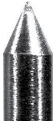
MultiStrike® Tungsten after 200+ welds
