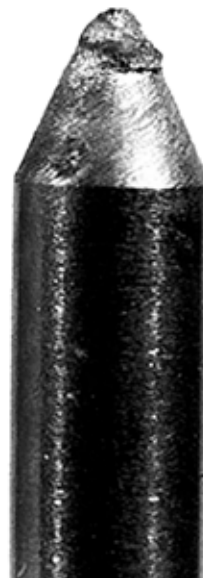
2% Thoriated Tungsten after 20 automatic welds
