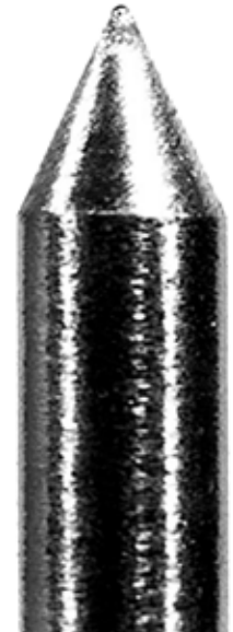
MultiStrike® Tungsten after 200+ welds
