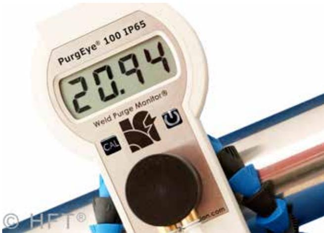
Before welding can begin, it is essential to know that the oxygen level at the weld zone has been reduced to an acceptably low level to achieve oxide free, zero colour welds.
