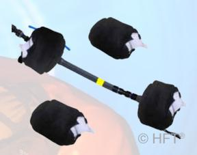
To fill the gap for smaller diameter pipework and for larger diameter pipework that doesn't justify the use of HotPurge™ Systems, HFT® have designed and manufactured Heat Covers for both PurgElite® and PurgExtra™ Tube and Pipe Weld Purging Systems with a temperature endurance of up to 300°C.
